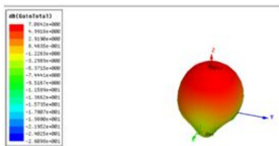
Figure 3.4 Gain for Three slot antennas using Roger RT/Duroid 5800 material
