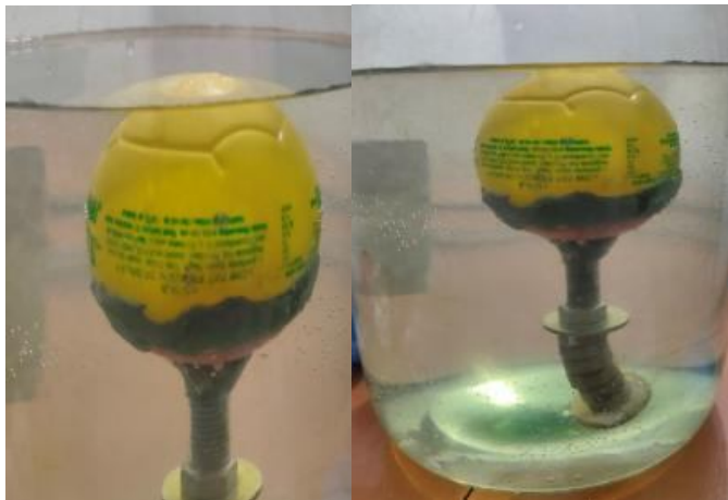
Figure 6: Circular body or ball in neutral buoyant condition by trial and error method.
