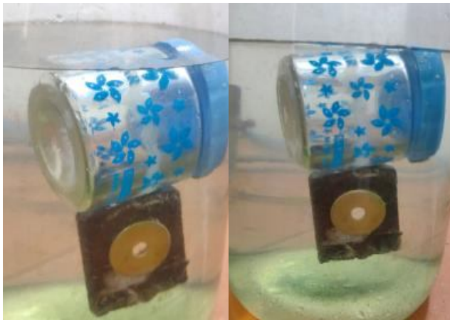
Figure 9: Cylindrical body in neutral buoyant condition by STEM design method.
