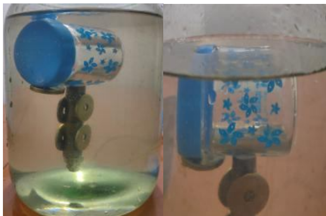
Figure 7: Cylindrical body in neutral buoyant condition by trial and error method.
