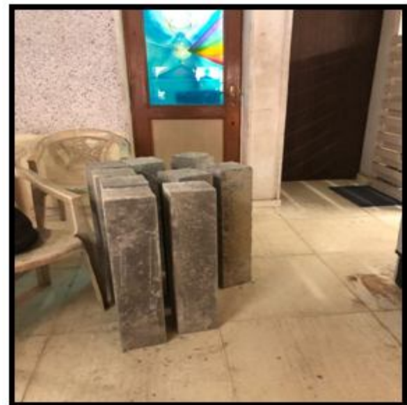
Figure: 2 M30 Grade concrete beam
