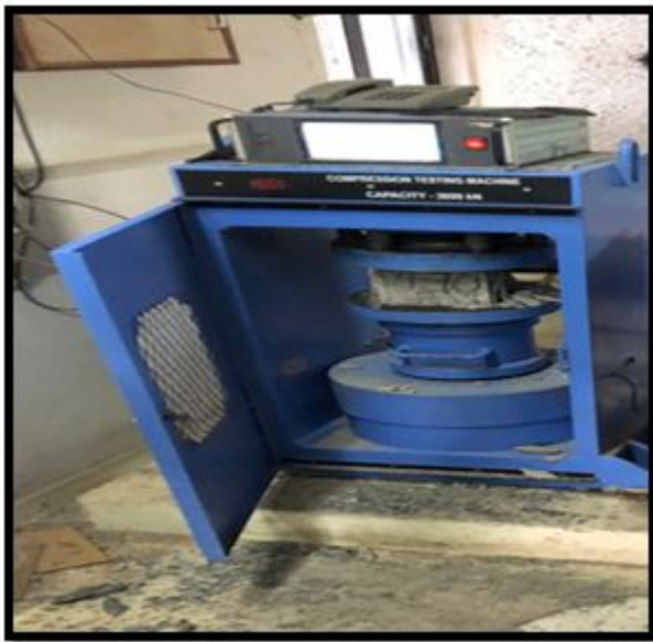
Figure: 3 Testing of M30 grade of concrete
