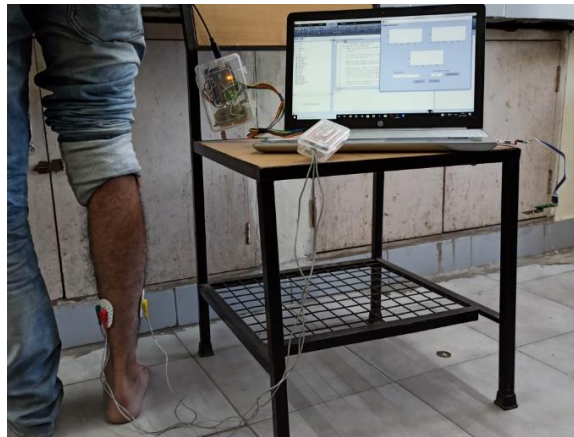
Fig. 1 EMG SET UP FOR RECORDING
