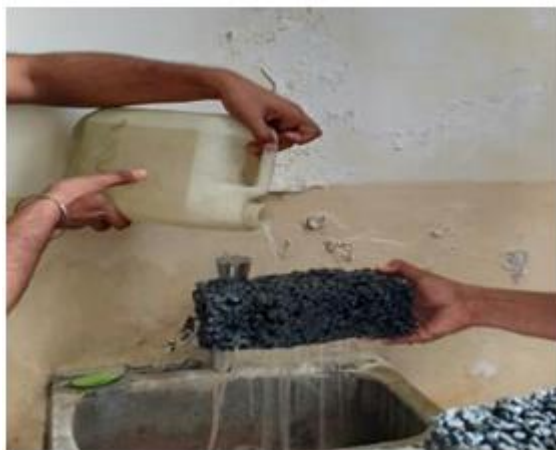
Fig. 3. Laboratory preparation & Permeability testing of Pervious concrete
