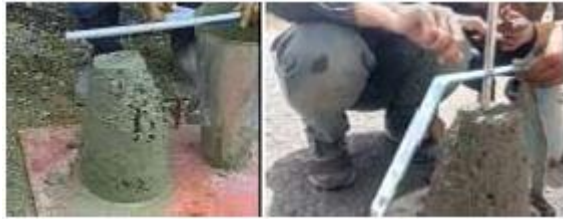
Fig -5: Slump cone for RMC & HMC
