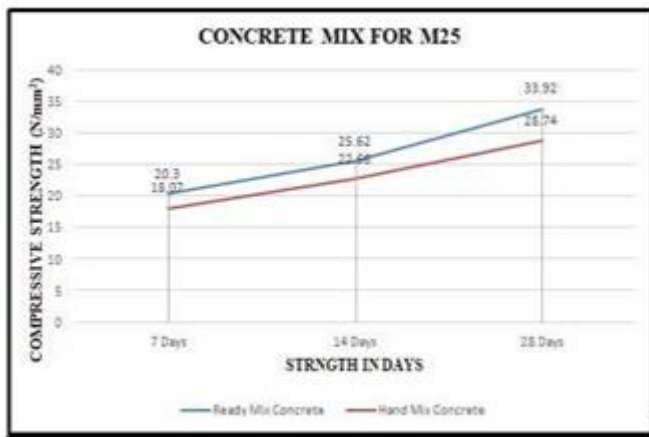
Fig -9: Graph showing comparison of RMC & HMC
