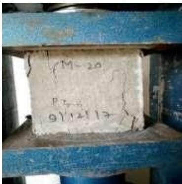
Fig -6: Compression Test in CTM
