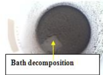
Fig. 1.5 Electroless nickel bath decomposition
