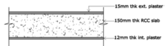
Figure 6 conventional RCC roof
