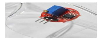
The eye-blink sensor works by illuminating the eye and eyelid area with infrared light, then monitoring the changes in the reflected light using a phototransistor and differentiator circuit. Here we used this sensor for Anti-sleep system.
