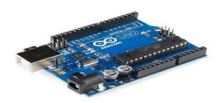
The Arduino Uno is an open-source microcontroller board based on the Microchip ATmega328P microcontroller and developed by Arduino.cc. The board has 14 digital I/O pins (six capable of PWM output), 6 analog I/O pins, and is programmable with the Arduino IDE (Integrated Development Environment), via a type B USB cable. It can be powered by the USB cable or by an external 9-volt battery, though it accepts voltages between 7 and 20 volts.
