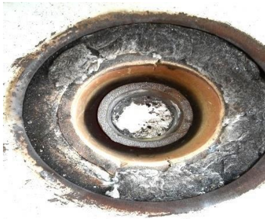
Melting of Aluminium in a Furnace
