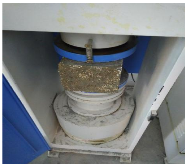
Figure 3.1 - Test Setup of Compressive experimental work
