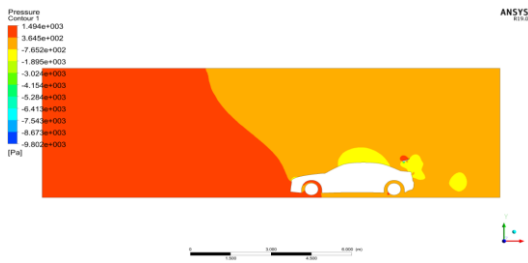
Figure: 5.5 Car with spoiler at angle -15 degrees
