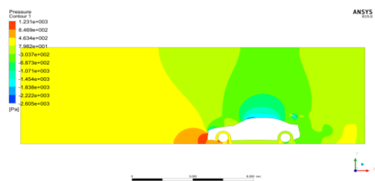
Figure:5.4 Car with spoiler at angle 30 degrees
