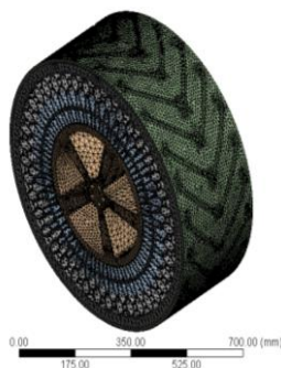
Fig 6 Meshing of the Geometry consider
