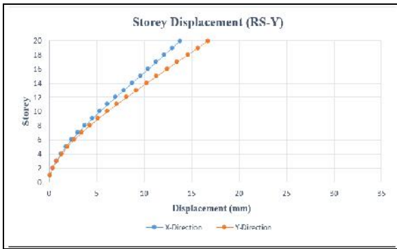
Fig. 18 Storey displacement in RS (Y-direction)
