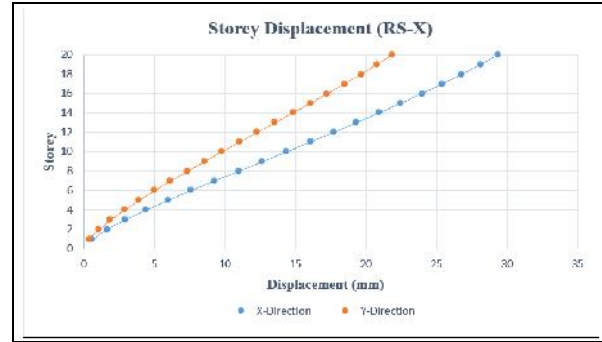
Fig. 5 Storey displacement in RS (X-direction)
