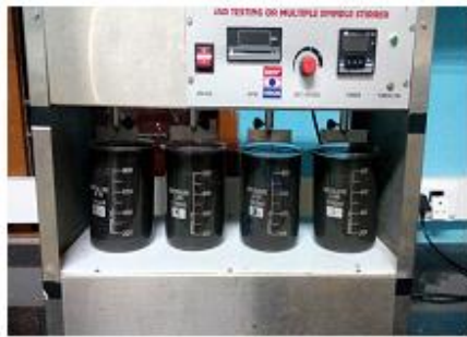
Fig. 4. Coagulation and Flocculation process Using Multiple spindle stirrer
