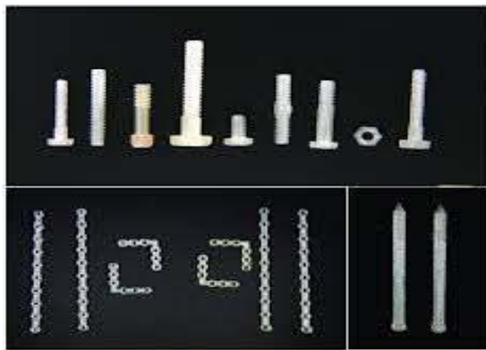
Figure 5: 3D printed PLA orthopaedic screws
