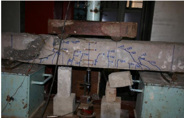
Fig.3.1 Load Propagation and Crack Pattern of H-RCB1
