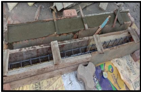
Figure 2.2 Casting of specimen
