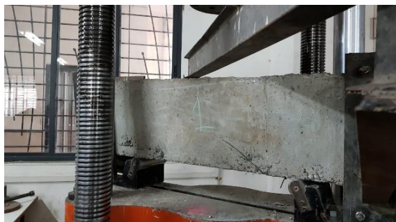
Figure 2.3 Pre- retrofitting loading
