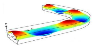
A wave guide detects light by surrounding a guiding region known as the core, made from a material with index of refraction n(core). Most waveguides are non-planar.
