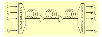
Optical communication of information having data rate higher than 10 Gbit/s is achieved using a popular technique which is known as wavelength division multiplexing (WDM). Several signals with different wavelength are sent through the same optical fiber using this technique.
