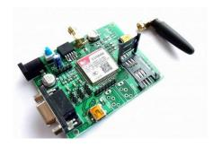
The SIM800 delivers GSM performance for voice, SMS, Data with low power consumption. It has one UART port, one USB port which is for updating firmware and for error detection. It has an operating voltage ranging between 3V to 5V. SIM cards can be inserted in GSM module. Our SIM cards are first registered in the core part of GSM which is the mobile switching center. This mobile switching center is
