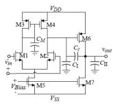
Figure 3: Miller compensated two stage op amp
