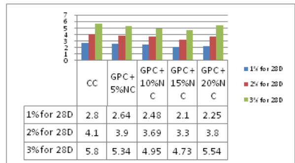
Compressive strengths of Nylon Crystal cube specimens with H2SO4
