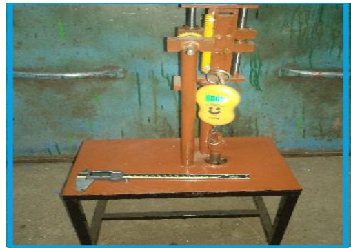
FIG. 1 TEST RIG FOR TEST ON SPUR RACK BY FDM PLASTIC MOULDING PROCESS
