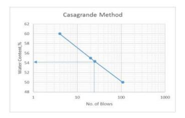
Liquid limit as obtained from graph = **52.33%** (corresponding to 25 blows)
