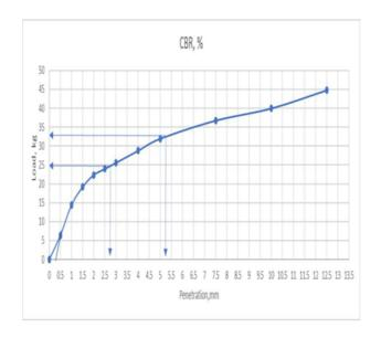
Load as obtained from graph at 2.5 mm penetration = 25 kg, CBR of Specimen = (25/1370) \*100=1.812%Load as obtained from graph at 5 mm penetration = 34 kg CBR of Specimen = (34/2055) \*100=1.645%
