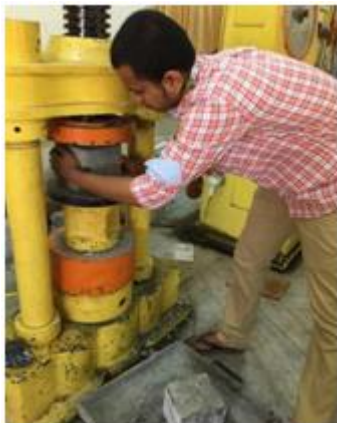
COMPRESSIVE STRENGTH TEST
