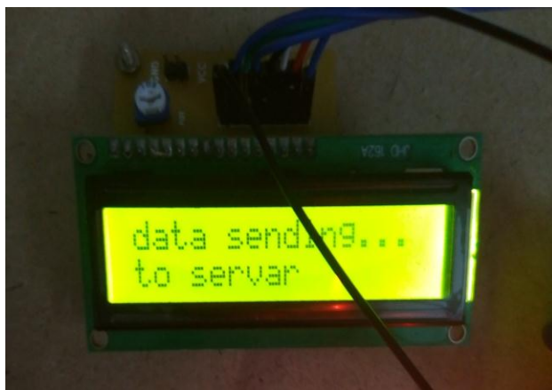
Fig : Data is uploading in server shown in LCD display.
