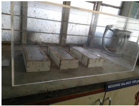
Fig. 7 Specimen placing in the environmental chamber just after the casting in moulds.
