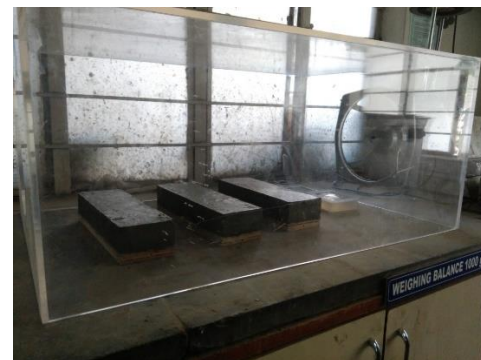
Fig. 5) Specimen demolding after 2-3 hrs. of casting
