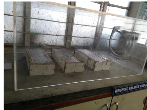
Fig. 4) Specimen placing in the environmental chamber just after the casting in moulds.
