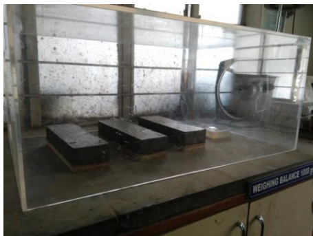
Fig. 8 Specimen demolding after 2 hrs. of casting
