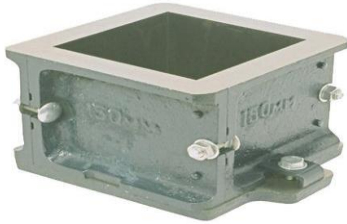
Fig: 4.2 Casting Mould (150x150x150) mm
