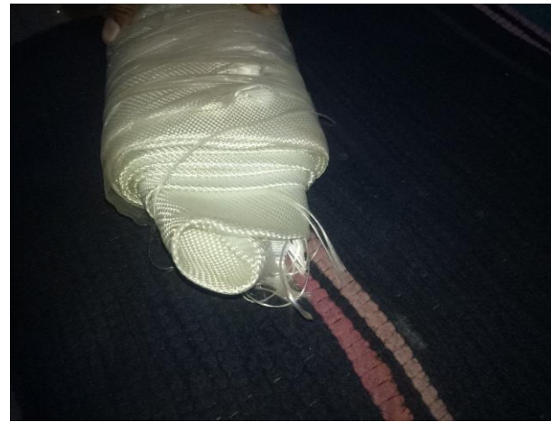
Figure.1 – Glass Fiber Reinforced Polymer Sheet
