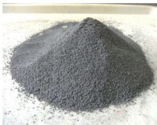
Fig 3.3: Black and glassy colour Aluminium slag
