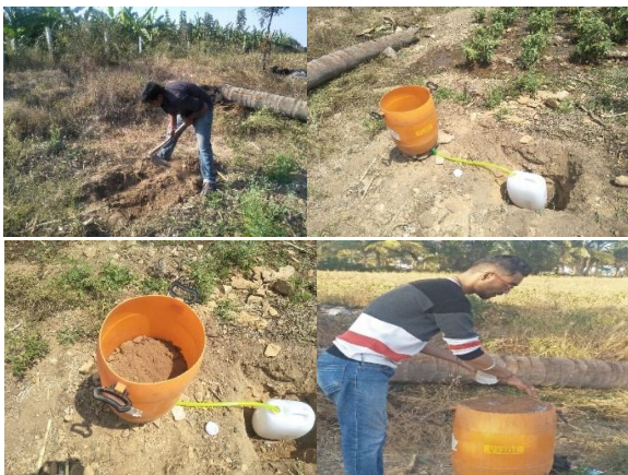
Fig. No.1 Installation of Lysimeter on Site.
