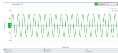
Fig. 8. Filter Stage I Simulation Circuit Waveform 10Hz Input Courtesy SIVANANDA ELECTRONICS Reprinted By Permission
