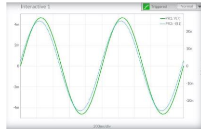
Fig. 3. Current to Voltage and Amplier Stage I Simulation Circuit Waveform Courtesy SIVANANDA ELECTRONICS Reprinted By
