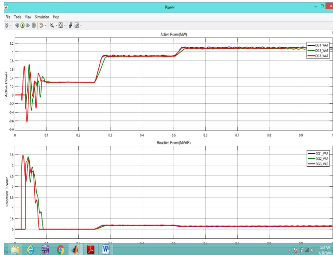
Fig 4(a): Simulation results for DG1,DG2 ,DG3 (a) Output active power. (b) Output reactive power.
