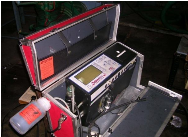
Figure 4: MRU Emission Monitoring System
