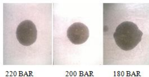
Fig 11: Spray Pattern Of B30 Biodiesel For Different Nozzle Pressures
