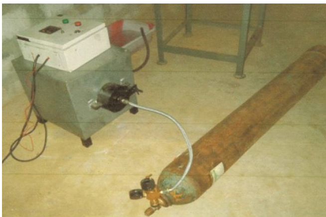
Figure 2: Sintering furnace used in this project.
