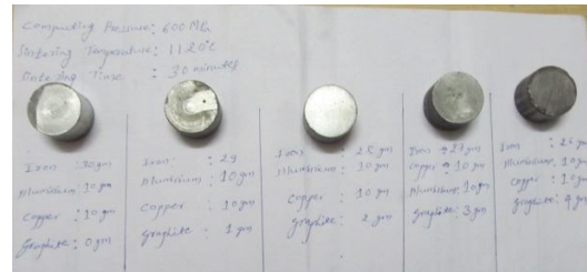
Figure 3: Components manufactured through powder metallurgy technique, here components from left to right refer to components containing 0% graphite,2% graphite,4% graphite,6 % graphite and 8% graphite respectively.
