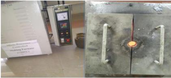
Fig 3.1 Laboratory casting set up
