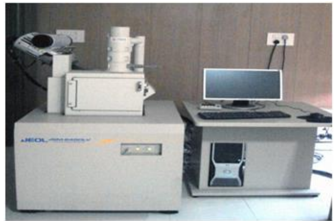
Figure 3.2 JEOL JSM-6480LV scanning electron microscope
