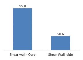
As far as Story Displacement is concerned, it is observed more in case of shear wall at core. This is due to in model 2 four shear wall at corners are provided. It increases rigidity of building and ultimately stiffness of building.
