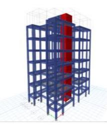
**Model 2:** Symmetrical building with shear wall at sides. A G+8 multi-storey building with shear wall is analysed with same loading conditions and materials. Shear wall location is considered as variable whereas other parameters used as constants.
