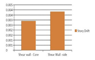
Story drift is another significant structural parameter. Building with shear wall at sides show more drift as compared to building with shear wall at core.
