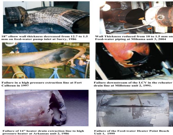
Fig 1. Examples of failures due to FAC worldwide
