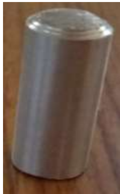
Fig-8: Specimen for Compression test as per ASTM-E8-13mm×26mm
