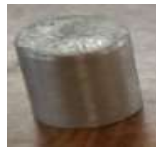
Fig-12: Specimen for Surface Micro Structure test as per ASTM-E8-18mm×18mm
