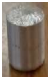
Fig-10: Specimen for Density test as per ASTM-E8-10mm×10mm
