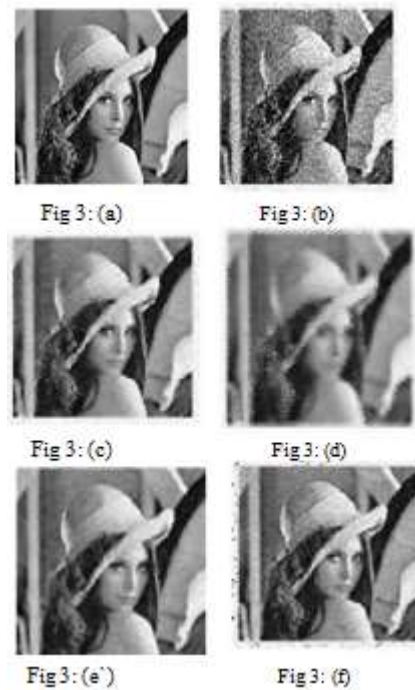
(a) Original image (b) Noisy image (c) Wiener and Wavelet (d) Haar and ATMAV (e) ATMAV and Haar (f) Haar and ATMED
