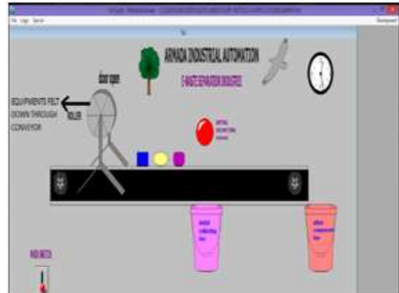
Fig:15 Roller Roating For 20seconds and Door open downwards the equipments are send through the conveyor in SCADA
