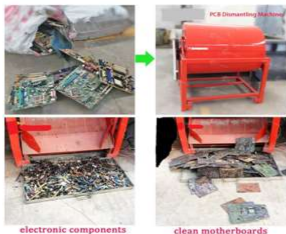
Fig:6 Dismantling of PCBs
