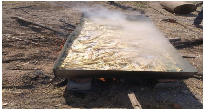
Figure: 3.2 Boiling of bagasse fibers The samples were then dried under the sunlight. Finally, samples were subjected to chemical extraction.
