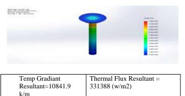
5.2.2 Closed condition @ 558 Temp Kelvin with Tail EN52 & Head Titanium carbide
