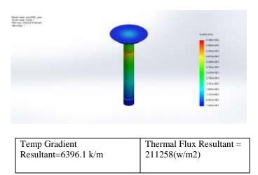
6.1.3 Closed condition @ 560 Temp Kelvin with Tail EN52 & Head Titanium Carbide.
