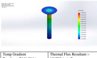
Resultant=7441.88 k/m 156280 (w/m2) 6.1.2 Closed condition @ 560 Temp Kelvin with Tail EN52 & Head Silicon Chromium Steel.
