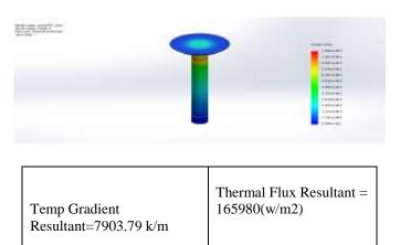
6.1.5 Open condition @ 578 Temp Kelvin with Tail EN52 & Head Silicon Chromium Steel.
