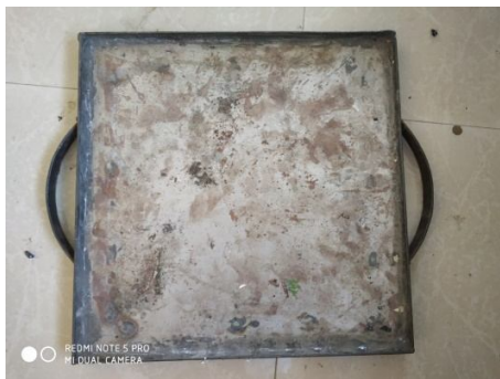
Figure 1 Mould for casting of plastic tiles
