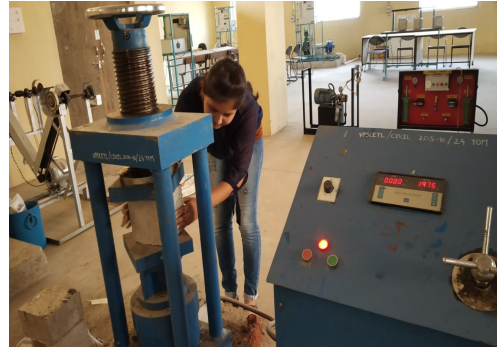
Fig. 3 Compressive strength test setup
