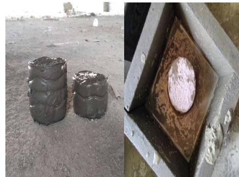
Fig. 5 Formation of specimen with demolished materials and placing in cube.
