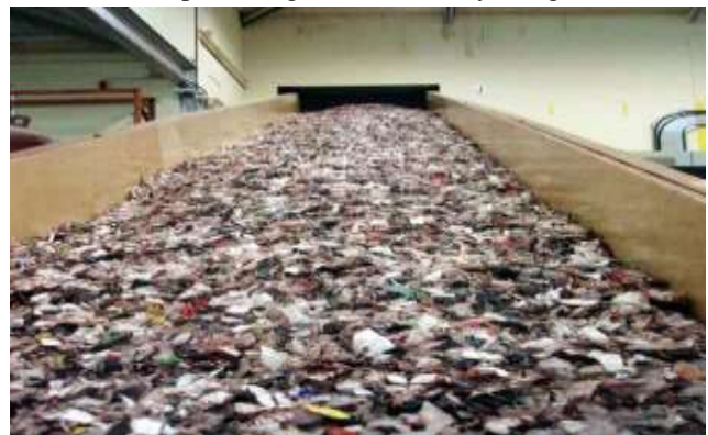
Fig.No. 3. Mixing of shredded waste plastic.
