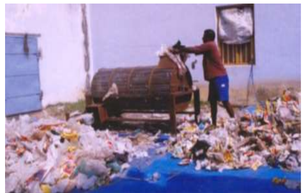
Fig.No. 2. Cleaning and shredding of waste
