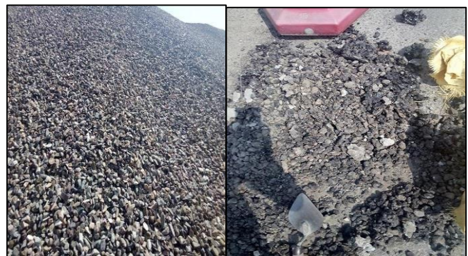
Figure 1.1 Natural aggregate and aggregate for recycle(waste)
