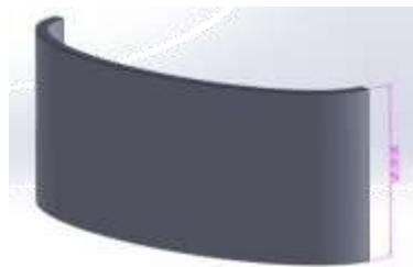
Fig. 2: Curved Rectangular Winglet (CRW)
