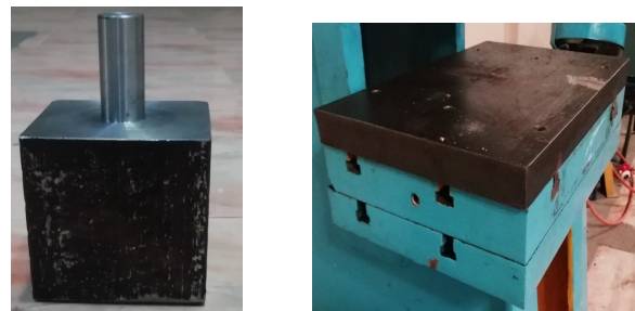
Fig 3 shows Fabrication of Base plate and Top die Design
