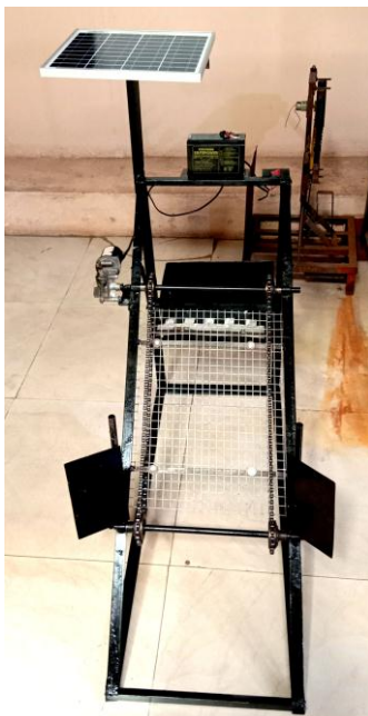
Fig: Fabricated “Solar powered drainage cleaning system”
